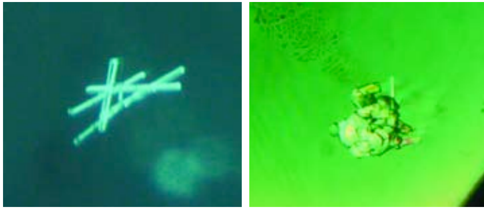
Figure 6. These images show examples of inclusion aggregates formed by transparent colorless prismatic crystals in Malossi synthetic emeralds. Their optical characteristics and occurrence in hydrothermal synthetic emerald suggest they are phenakite. Photomicrographs by Renata Marcon, in darkfield illumination (left, magnified 100 \times ) and with crossed polarizers (right, magnified 50 \times ).
